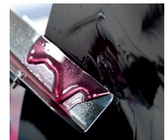
Abstreifung in die Ablaufrinne Stripping in the drain trough
